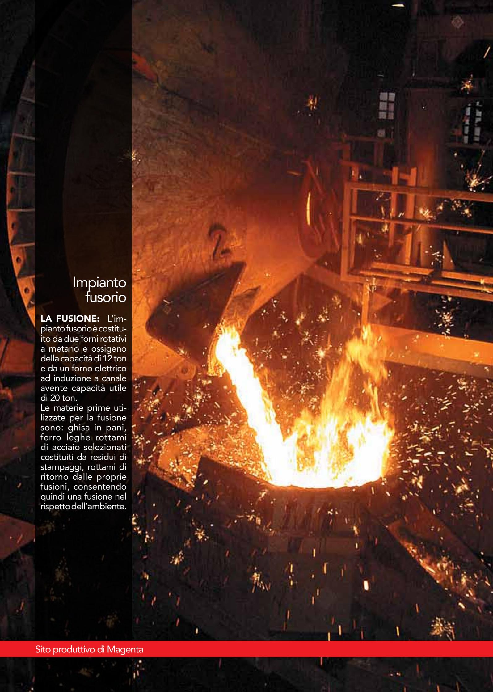
A large industrial ladle is tilted, pouring a thick stream of bright orange molten metal into a furnace. The scene is filled with intense heat and a shower of bright sparks falling from the point of contact. The background shows the dark, industrial interior of a steel mill with some structural elements and windows.
